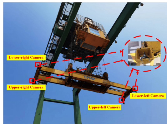
Fig. 1. The cameras mounted on the RTG crane spreader
