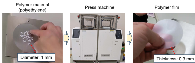
Fig. 3. Producing process of film specimen of polymers by heat pressing
