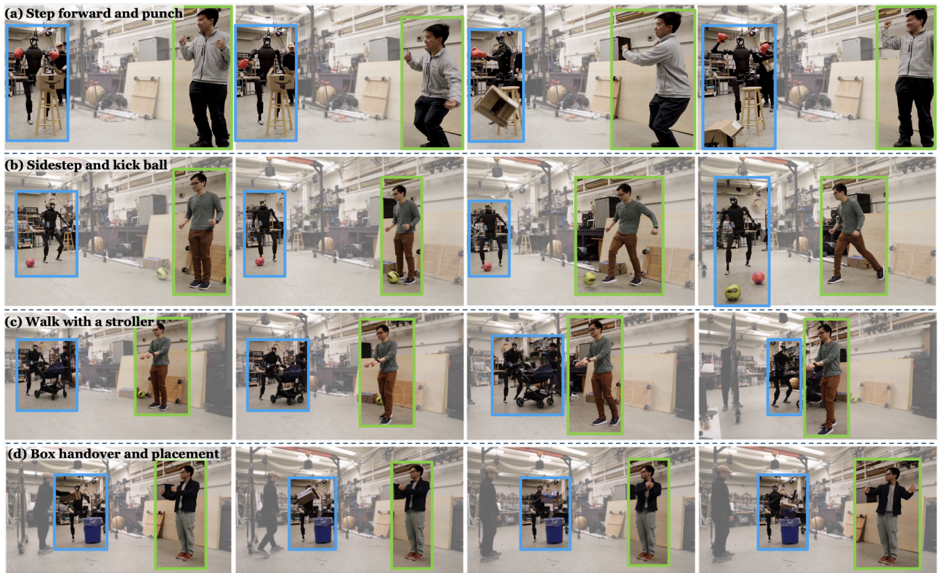
Fig. 1: The humanoid robot is teleoperated in real-time using an RGB camera by the human teleoperator . (a) The humanoid mimics the human teleoperator, advancing one step while delivering a punch to displace a box, followed by a victory gesture. (b) The humanoid executes a precise sidestep to align with a ball and delivers a controlled kick using its right foot. (c) The humanoid demonstrates forward walking while pushing a stroller. (d) The operator teleoperates the humanoid to catch a box, rotate its waist, and drop the box into a waste bin. Videos: see the website .
