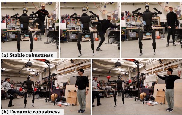
Fig. 7: Robustness Tests of our H 2 O system under powerful kicking. The policy is able to maintain balance for both stable and dynamic teleoperated motions.
