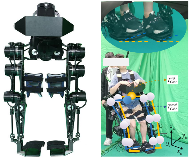
Fig. 1. The developed lower limb exoskeleton, close-up view (left) and the user wearing the exoskeleton (right). The yellow link represents the ideal rigid body state, while the blue link represents the actual exoskeleton state. Videos can be accessed online [33].
