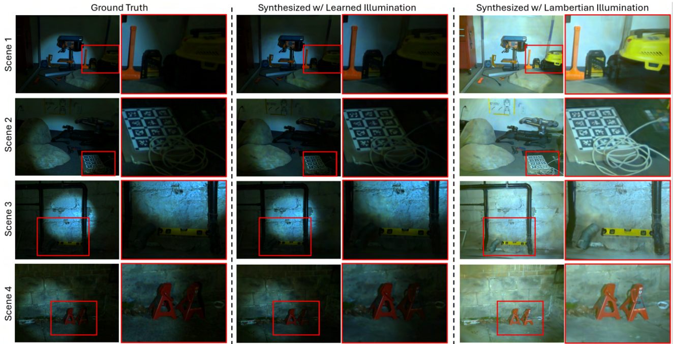
Fig. 8: Visualization of results from multiple scenes: We show that with DarkGS, we can reconstruct the scene with RAW images from robotic deployments in dark environments, and relight the scene to reveal more information that is corrupted in the RAW image due to uneven and partial illumination. Results as shown are all from the flashlight setup which is the most challenging according to our numerical results.
