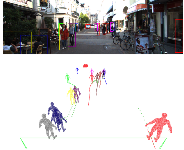
Fig. 1: A brief overview of our perception system's output: the top image shows an RGB frame, while the bottom image depicts the corresponding perception result. It includes reconstructed moving objects, color-coded for classification, with their predicted trajectories marked by green dashes.
