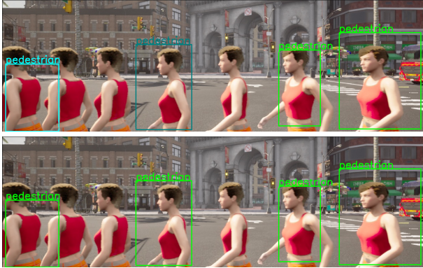
Fig. 7: Comparison between original QD-3DT (top) and our proposed method (bottom). The person in the red shirt is the same person in a different time step.
