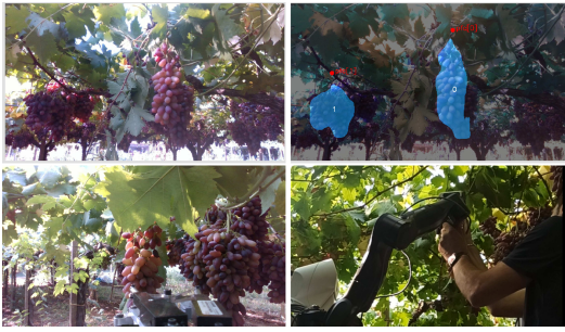
Fig. 6. Top Left: image of the grapes from the head camera of the robot. Top Right: grapes recognition and peduncle localization. Bottom left: images of grapes taken from the right wrist camera. Bottom Right: human assisting the robot for grape harvesting.
