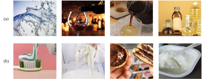
Fig. 1: (a) Newtonian fluids: distilled water, red wine, black coffee, and cooking oil. Despite their varied molecular structures, fluids in (a) consistently obey Newtonian principles. (b) Non-Newtonian fluids and their properties: toothpaste (Bingham plasticity), Oobleck (shear-thickening, impact resistance), chocolate sauce (thixotropy), and Bulgarian yogurt (viscoelasticity).
