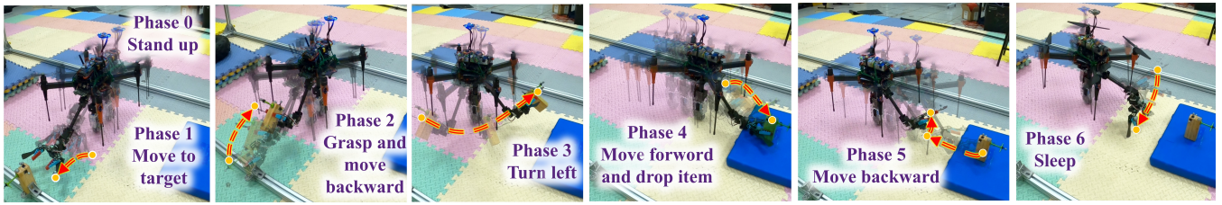
Fig. 5: The time-lapse photos of the manipulation experiment. The yellow points and red arrows illustrate the movement of the end effector.
