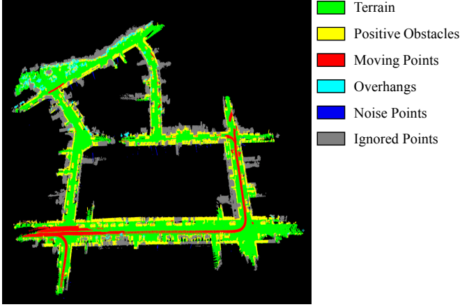
Fig. 5. By applying the terrain modeling and moving point identification method proposed in [27], we can classify each point in SemanticKITTI sequence 07 into ignored, noise, terrain, positive obstacle, and overhang.
