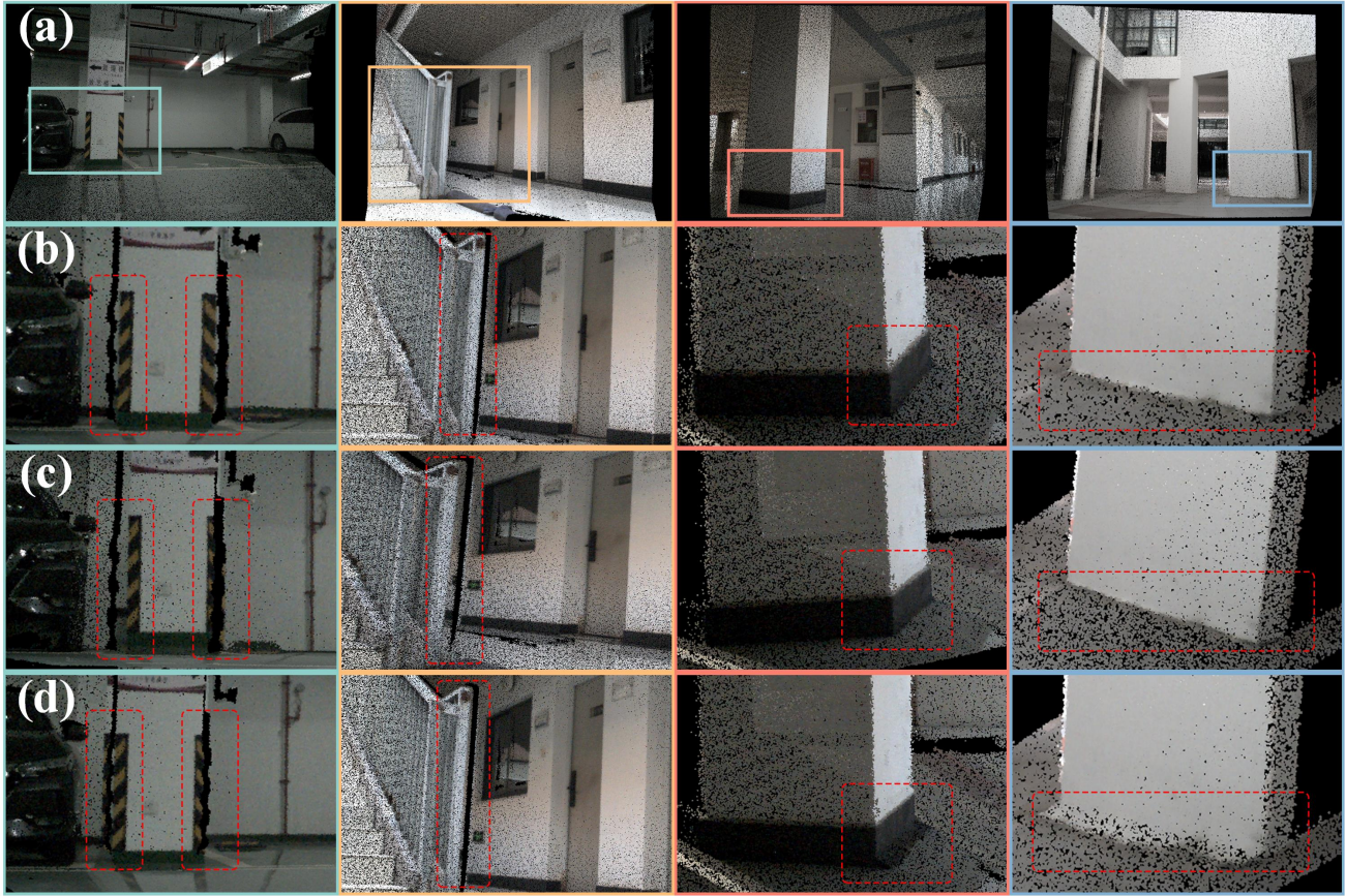
Fig. 9. (a) Colorized point clouds using “pseudo” ground-truth calibration parameters, with the area within the square frame designated for comparison. (b) The result of colorizing with our calibration result. (c) The result of colorizing with Yuan’s calibration result. (d) The result of colorizing with Koide’s calibration result. The red boxes emphasize areas with noticeable differences in color alignment.
