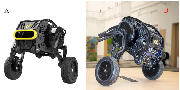
Fig. 1: A novel 6-DoF wheeled bipedal robot composed entirely of direct-drive joints. (A) DIABLO keeping balance on flat ground. (B) DIABLO maintaining balance involving body tilt and non-horizontal orientation of the head. Accompanying video is available at https://youtu.be/mm0XruFvZ4U
