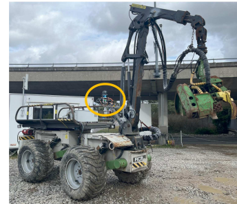
Fig. 6: SAHA in a construction site, the yellow circle indicates the vehicle-mounted LiDAR.
