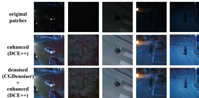
Fig. 7. Visualization of the denoising effect of CGDenoiser functioning on enhanced frames. Apparently, images after enhancement are seriously degraded by intricate real noise. With denoising support from CGDenoiser, the quality of frames recovers conspicuously.
