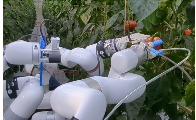
Fig. 1: HortiBot: A three-arm system with active perception and dual-arm manipulation for robotic horticulture. The right arm is used for grasping, the left arm performs cutting, and the central arm moves stereo cameras for mapping and online observation.
