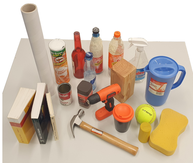
Fig. 4. The object set used for training, testing, and evaluating the approaches. It comprises 20 differently shaped objects of various sizes and strengths, partly from the YCB object set [21]. Each object was grasped three times.
