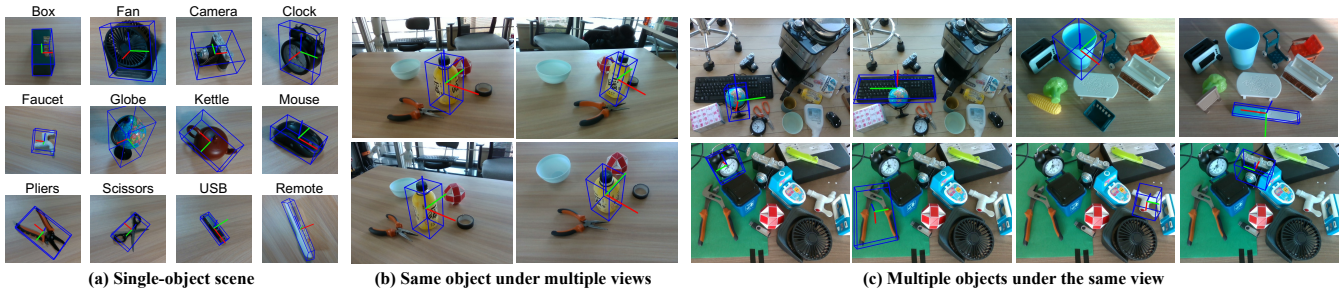
Fig. 4. Results of real-world object pose estimation. (a) Test results of single-object scene. We present a subset of the visualization results of the pose and size estimation using the trained MVPoseNet6D model. The outcomes are represented with a tightly oriented 3D bounding box and colored XYZ-axis. (b) The scene with same object under multiple views. We show the pose of a bottle under different views. (c) The scene with multiple objects under the same view. We show the pose estimation of different objects in several cluttered scenes.
