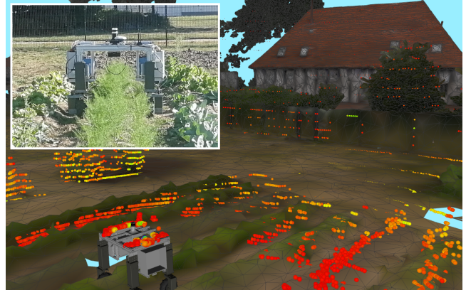
Fig. 1: The Lero agricultural monitoring robot uses MICP-L for localization for mesh-based navigation between beds in a market garden micro-farming environment.
