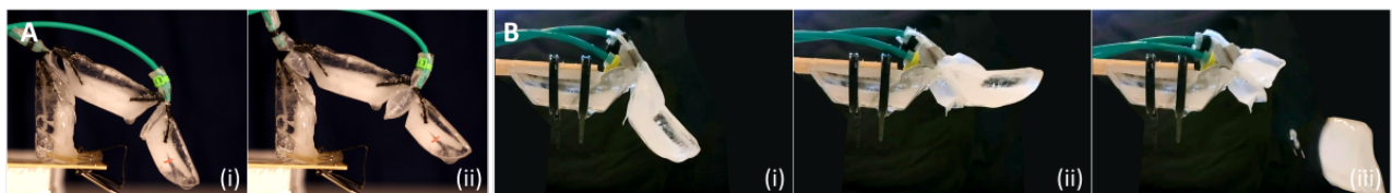
Fig. 6. A) 3-link robot finger, composed of ice links and 2 pouch motors which also serve as flexible joints to hold the links together. B) 2-link robot finger, shedding its outer link by over-inflating the corresponding pouch motor to produce an ice fracture.
