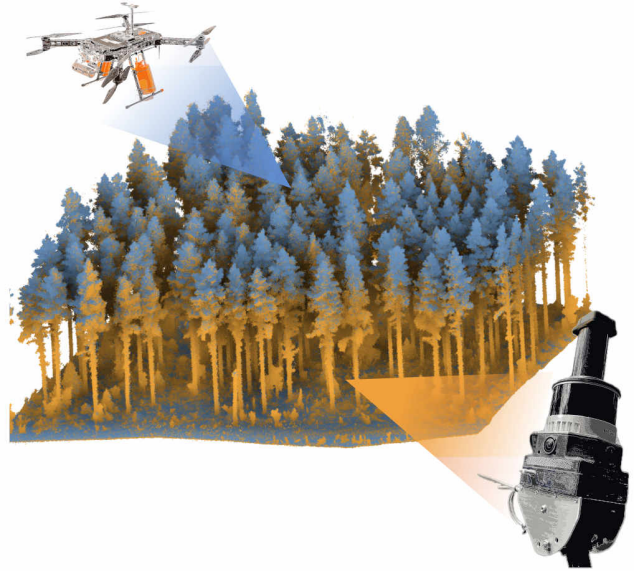
Fig. 1: A forest map built using a terrestrial map from our mobile scanning system (orange) and an aerial map from a drone (blue). Together, the scans produce a map reconstructing the canopy and understory in sufficient detail for individual-tree forest inventory.
