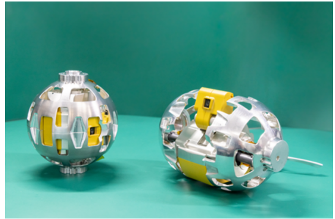
Fig. 2. Photograph of LEV-2s in the folded and transformed shapes. Courtesy of the JAXA/TOMY Company/Sony Group Corporation/Doshisha University.
