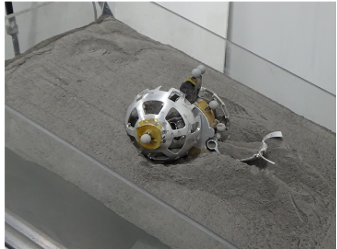
Fig. 9. Photograph of the LEV-2 EM in the slope traveling test. LEV-2 traveled in the crawl mode over a sloped terrain.
