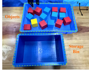
Fig. 2. (Left) Methodology for packing with different constraint and contact states. Reds represent the eight cubes in corners, blues denote the middle six cubes with already packed objects on both sides, and the yellow one is the last cube to be inserted. The constraint surfaces are the reliable conditions to maintain compactness, and the contact surfaces represent the directions of errors and contact with other objects. (Right) The initial configuration of the packing task.
