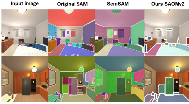
Fig. 3. Comparison between vanilla SAM, Semantic SAM and our SAOMv2 on images from Ai2Thor simulator in the “everything” mode. SAOMv2 predicts the instance-level object masks for both the background and the foreground objects, while SAM tends to divide background objects on parts and sub-parts.
