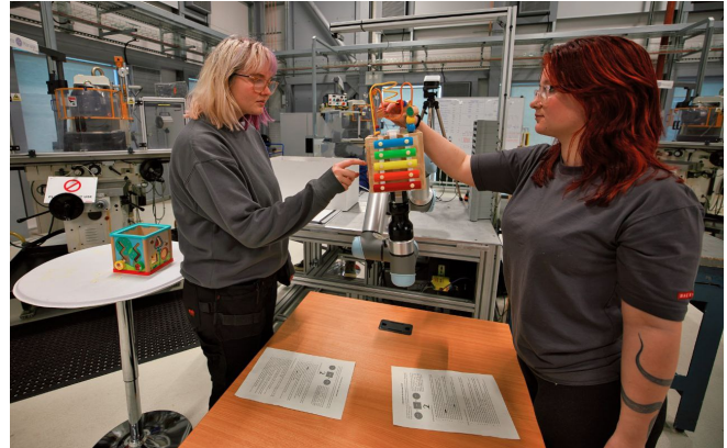
Fig. 1. Experimental setup of the multi-user human-robot collaboration explored. The users need to perform different operations at the same time on a shared target object. The robot adjusts position and orientation of the object according to the progression of the interaction. Behind the user on the right, there was another table with a box on it (see Subsection III-A).
