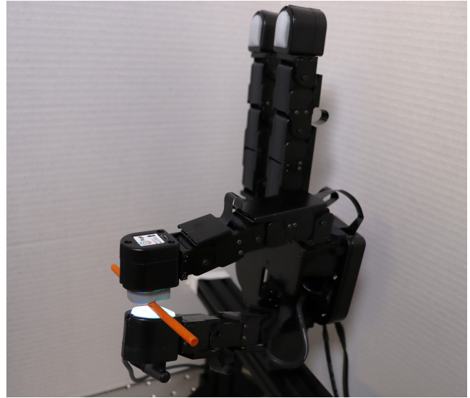
Fig. 1. The hardware setup for this work. Two fingers of the Allegro robotic hand are used to manipulate a piece of stick. The Digit vision-based tactile sensor on the thumb finger reads the contact state and enables manipulation without visual feedback
