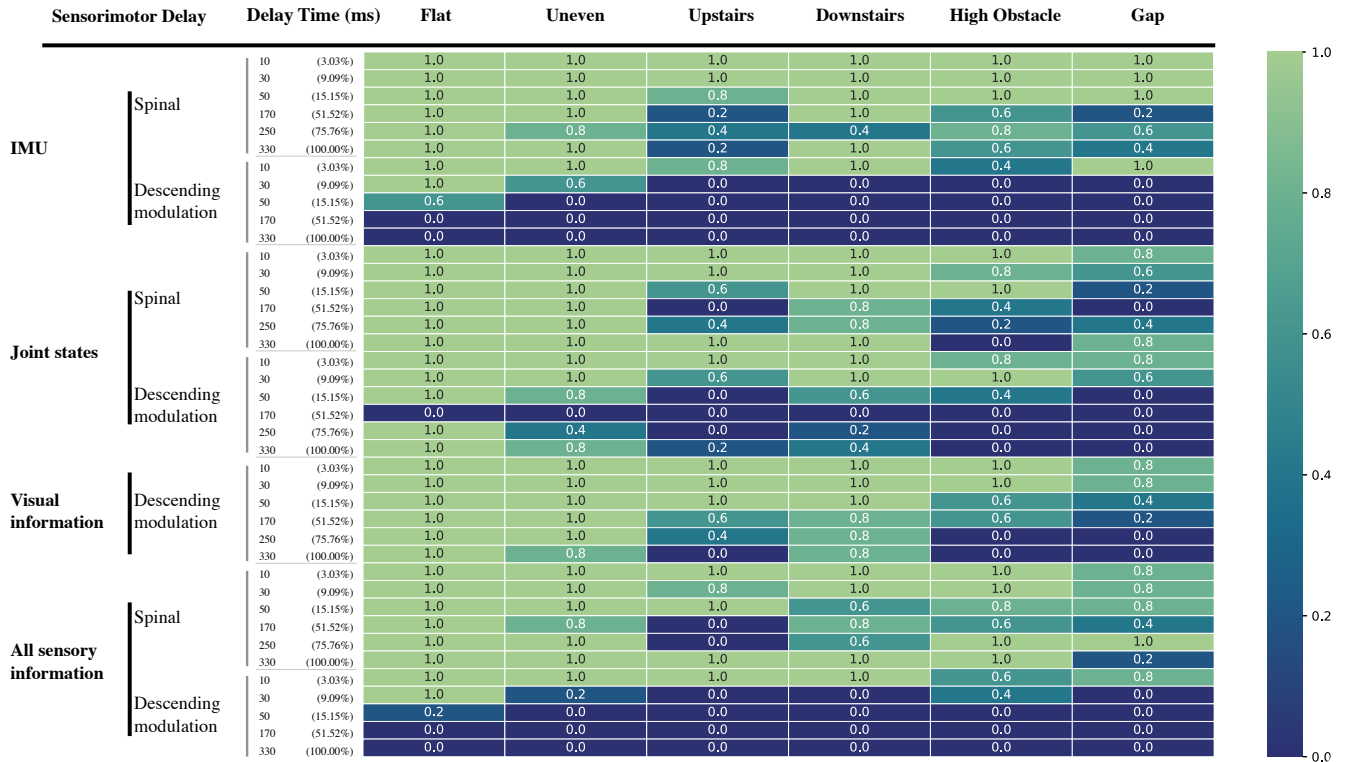
Fig. 5. Success rates for sensorimotor delay experiments: The robot is commanded to travel at 0.9 m/s across six types of terrain—flat, uneven, upstairs, downstairs, high obstacles, and gaps. Each terrain tests the impact of varying sensory delays on two control policies: the spinal policy and the descending modulation policy. Each experiment involves five trials, activating both policies simultaneously, with the robot initiating each trial from distinct starting positions (for example, a success rate of 0.6 indicates three successes and two failures). It’s important to note that both policies tested were trained without sensorimotor delays. Additionally, the figure displays the delay time and its corresponding percentage of a single gait cycle.
