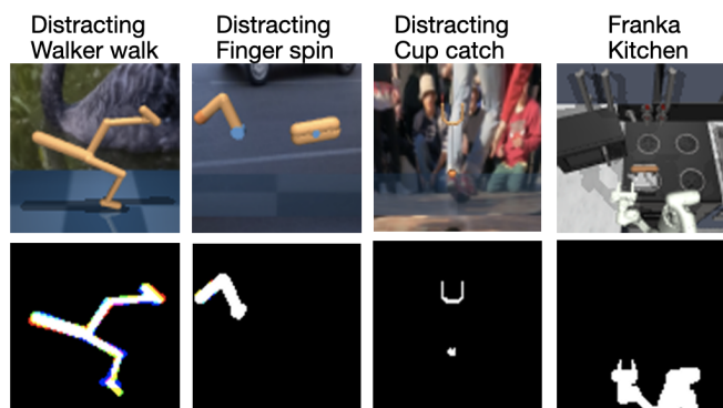
Fig. 4: Different environments used for validation. (top row) RGB images that are input to the agent (bottom row) agent segmentation masks.
