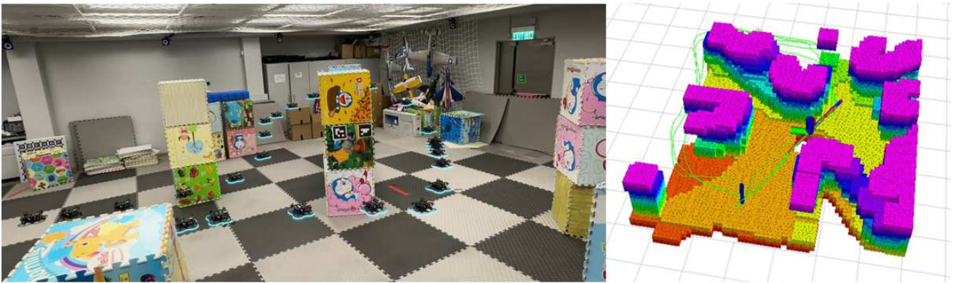
Fig. 9: Real-world autonomous navigation tests. Left : OmniNxt autonomously flies without rotating the yaw to the speed direction. Right : the executed trajectory and voxel map. (Sec. IV-C)
