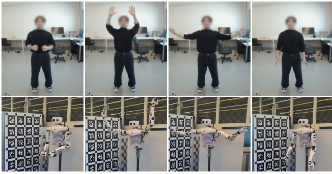
Fig. 5. Real-time retargeting of human poses from RGB images onto Reachy in a real world environment.
