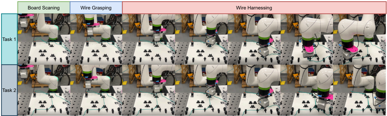
Fig. 7: Snapshots of the multi-wire harnessing task, where the robot needs to harness two wires in a sequence. The robot first captures the workspace point cloud to identify and grasp the wire. Then, the proposed harnessing motion is applied to align the wire to the fixtures. Task 1 and 2 represent two different desired wire shapes and are executed sequentially.
