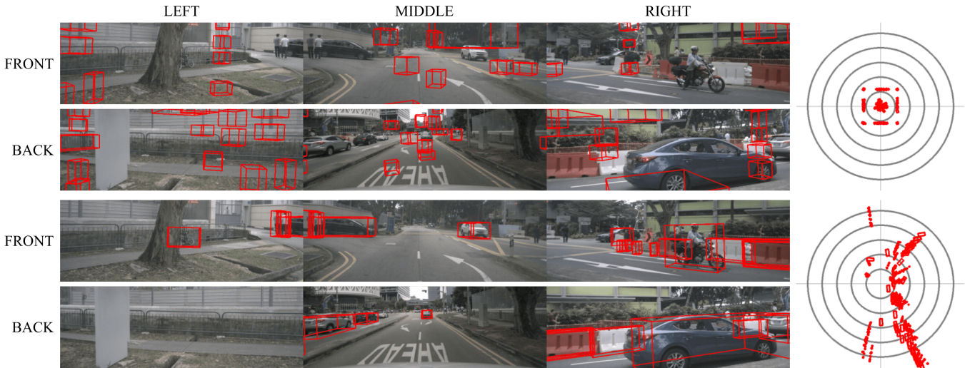
Fig. 5. Qualitative comparison between 3D proposals obtained from the learnable anchors setting (top) and our MDHA Anchor Encoder (bottom). We visualize selected proposals on all 6 cameras (left) and all proposals in bird’s-eye-view (right). For visual clarity, we display non-overlapping proposals for learnable anchors, and the top-20 proposals based on classification score for MDHA.
