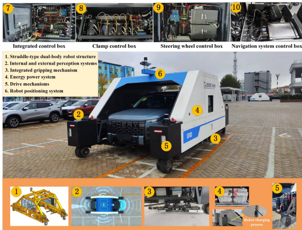
Fig. 1: The structure of the vehicle transfer robot system
