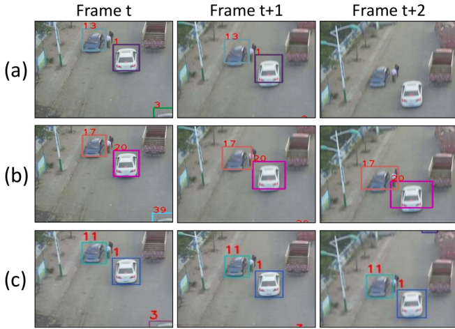
Fig. 2. Comparison of tracking results on a low-altitude video. (a) ByteTrack without motion-compensation (MC), fails to maintain tracks. (b) BoTSORT’s MC leads to distorted bounding boxes. (c) SFTrack with UAV MC, ensures consistent and accurate tracking.
