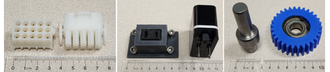
Fig. 5: Objects used in the experiments. From left to right, the objects are: AMP Connector PLUG (15-pin), AMP Connector HEADER, Power PLUG Adapter (NEMA 1-15P), Power PLUG Receptacle (NEMA 1-15R), Shaft (14.6 mm dia.), and Spur Gear (GEABDM2.0-30-20, 15 mm hole dia.).
