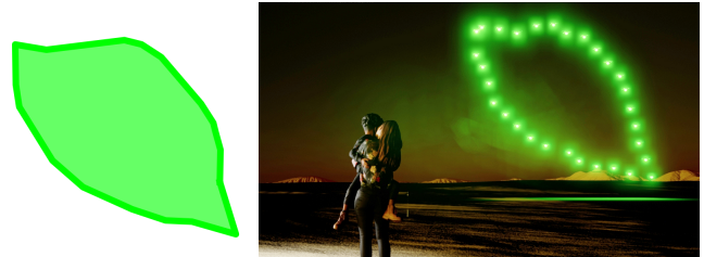
Fig. 1. Drone formation automatically crafted to match a given text. CLIPSwarm takes a single word describing a shape as input and automatically determines the color and positions of a robotic swarm formation that best fits the given text. The example illustrates the shape created by a formation of 30 robots. The drones move to positions that collectively form a shape corresponding to the word “Leaf”. Left: graphical representation of the shape formed by the robot formation. Right: formation of drones as part of a show in a photorealistic simulation representing the input word.
