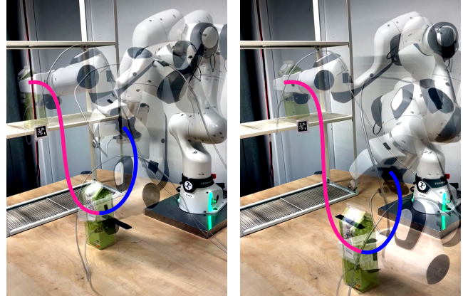
Fig. 1. In this work, we propose TPGP, a GP-based architecture to learn by demonstration tasks composed of multiple sub-tasks, like grasping and re-shelving objects. The two panels show two such executions.
