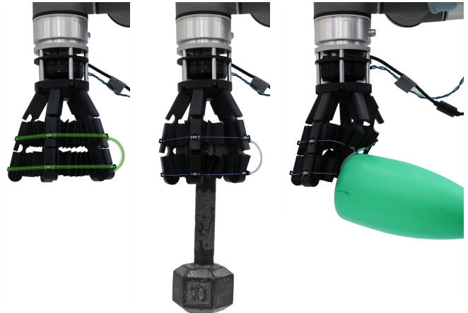
Fig. 1: Flexible Robust Observant Gripper (FROG) mounted on a Universal Robots UR5, with the cable path highlighted in green (left). FROG is simultaneously strong and compliant, shown lifting a 10 lb (4.5 kg) dumbbell (middle) and being deformed by a plastic bat (right).
