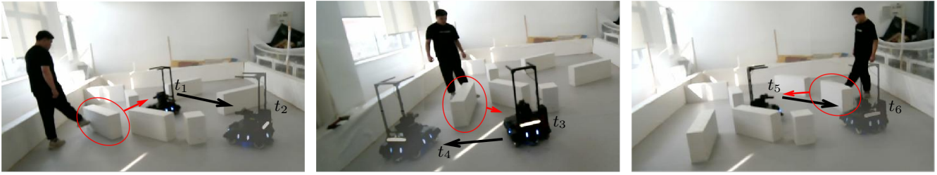
Fig. 9. The robot continuously tracks a person in a cluttered dynamic environment. At times t_1 , t_3 , and t_5 , the person moves obstacles (marked with red circles and arrows) to obstruct the robot's tracking, posing significant safety challenges to tracking. The robot senses changes in the environment, replans a new trajectory in real time, and avoids obstacles (marked with black arrows) while maintaining target visibility. The robot continuously tracks the target from t_1 to t_6 while ensuring trajectory safety, demonstrating the practicality of the SF-Tracker in extreme situations with safety challenges.
