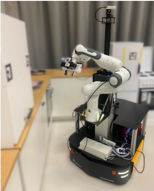
Fig. 3: Robot setup showing the Franka manipulator, with an end-of-arm depth camera, mounted onto a mobile base.
