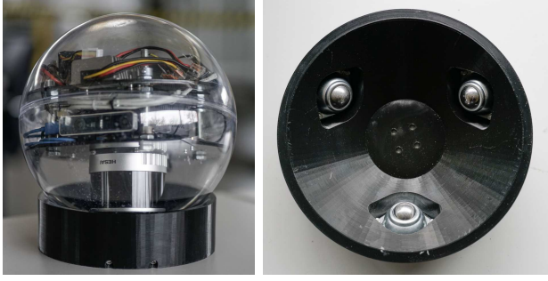
Fig. 3: Left: The spherical mobile mapping system housing a laser-scanner, IMUs, and an onboard computer inside the spherical protective shell. Right: 3D printed calibration apparatus needed to perform rotations of the spherical system without translation around the center point of the ball.
