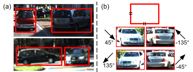
Fig. 6: (a) Variation in dimensional features of equidistant objects. Observe that box height remains almost identical, proving its robustness, whereas width and diagonal are affected. (b) Variation in allocentric orientation of equidistant objects with identical dimensional features, justifying the effective range reduction from [0, 360] to [0, 90] degrees
