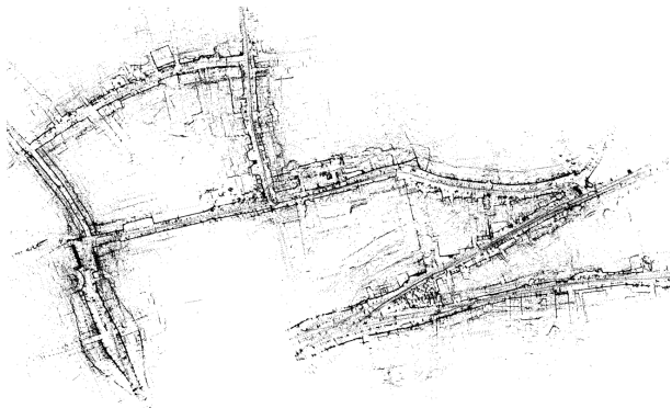
Fig. 1. Map obtained by testing the proposed method on partial sequence 10-14-35 of the Oxford Radar RobotCar dataset [12].
