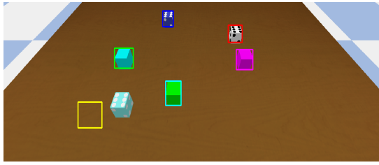
Fig. 6: Predictions of free-space pose prediction module. The task is to move the cyan lego to a collision-free position. The learnt module predicts collision free locations (yellow bounding box) from prior data. The learning accelerates the plan search by ameliorating the need for exhaustive enumeration of possible locations.
