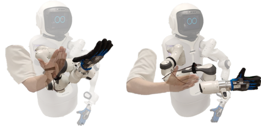
Fig. 1. Anthropomorphic arm mapping from human to humanoid robot.
