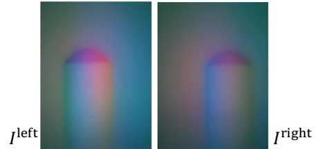
Fig. 6: Example tactile images when grasping a peg, which is inputted to the in-hand pose estimation model to estimate the grasp error and correct it before insertion.
