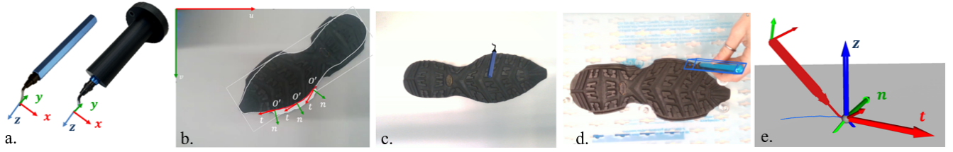
Fig. 4. a. Manual deburring tool and its 3D-printed support for robot installation. b. Local RFs T_{i,j}^{burr} = [t, n, z'] . c. BlenderProc generated image. d. EfficientPose prediction on one frame showing the operator executing the task. e. 3D reconstruction of the scene in d .
