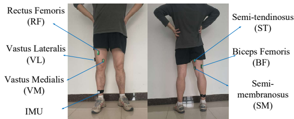
Fig 6. Collection of electromyography signals and joint angle signals.
