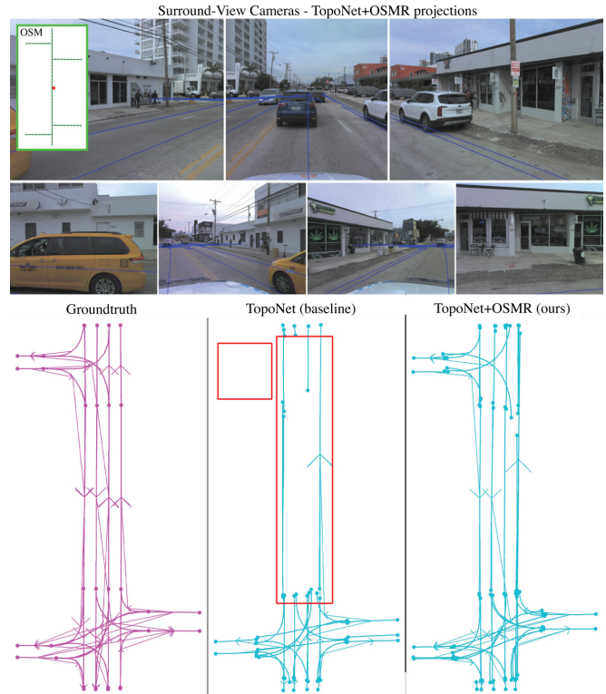
Fig. 1. Online road network perception and reasoning is challenging due to occlusion by on-road objects, especially at long-range as required by planning. In this example, the left turn map elements are heavily occluded by the vehicles. The baseline (TopoNet) using only image data misses the left turn while our method (TopoNet+OSMR—leveraging rasterized Standard Definition (SD) maps as the prior) predicts it correctly. Visualizations represent centerlines with connectivity information.
