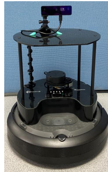
Figure 1. The Turtlebot4 with the modified camera mount position to provide a better field of view.
