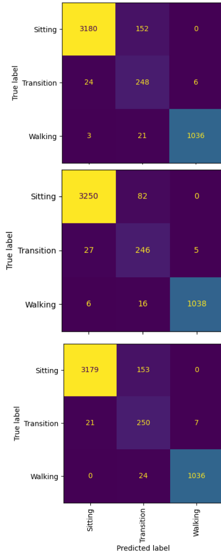
Figure 2. The confusion matrices for the SVM (Top), KNN (Mid) and RFC (Bottom) models on the labelled data. The x-axis labels represent the predictions and the y-axis represent the researcher's label.
