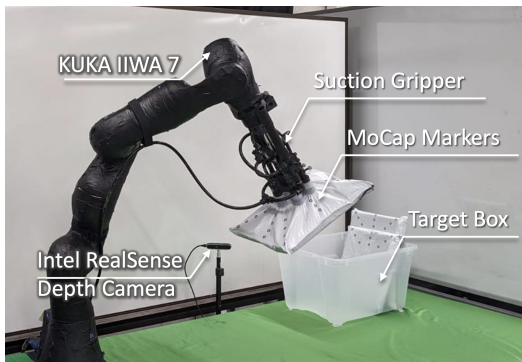
Fig. 3: Experimental cell showing manipulator with a suction gripper, used for package transport experiments during training and execution phases. MoCap cameras are not shown.
